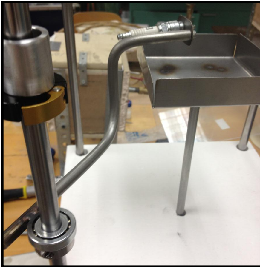
Figure 26. Spark ignitor mounting hardware.
