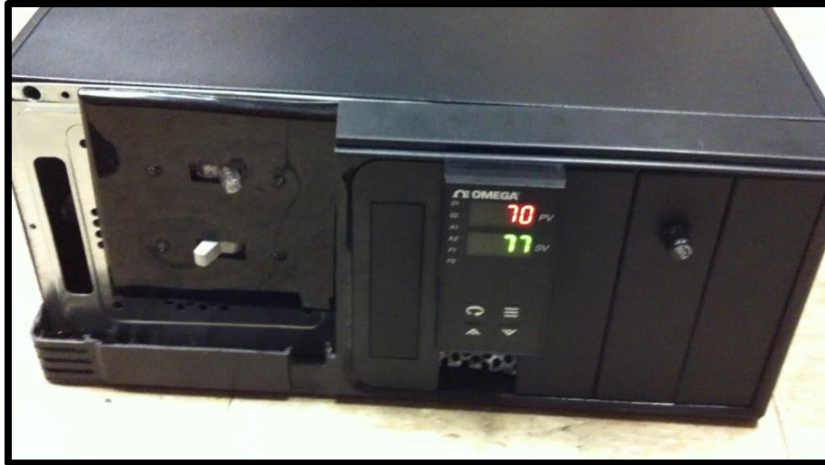
Figure 19. Control Tower operational. PV number represents Present Value for heat temperature. SV number represents Set Value for heater temperature.
