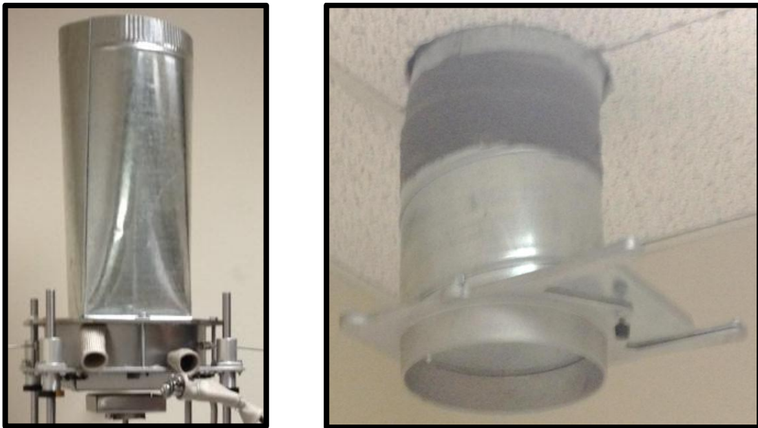
Figure 27. Left: Exhaust hood flange attached to the MLC. Right: Laboratory exhaust vent.
