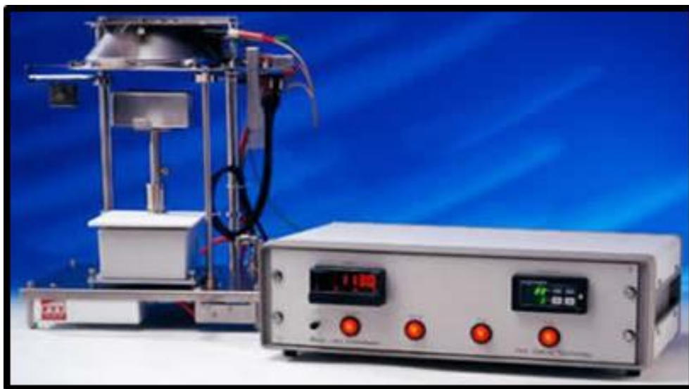
Figure 1. Commercially available mass loss calorimeter [5].
