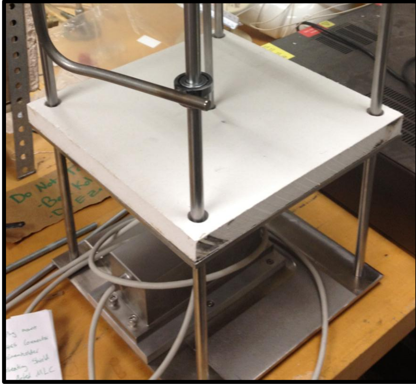
Figure 16. Shielding on middle plate to protect load cell.
